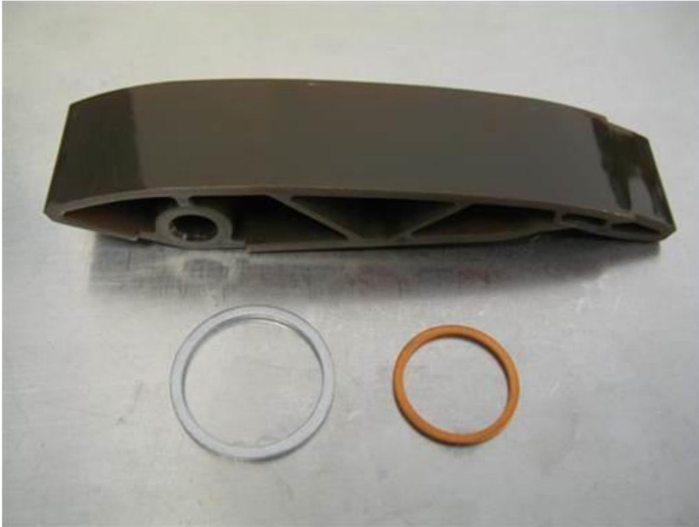
Exhaust upper chain tensioner guide (11-31-7-830-159) $16.83/each Chain guide mounting bolt washer (07-11-9-963-342) $1.11/each Crankshaft chain tensioner washer (07-11-9-963-418) $1.04/each
